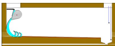
3. Once the self-tipping cleaner-bucket is filled, the point of gravity of the water-cleaning unit is displaced, causing it to overturn, instantly freeing the volume of water contained. The wave created sweeps the sediment deposited at the bottom of the tank, dragging it to a receptor channel.
