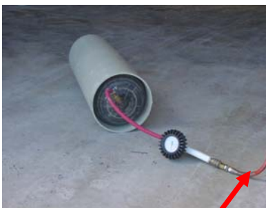
Conectar a compresor
