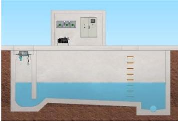
1.- The storm begins. A combination of wastewater and rain begins to fill the retention chamber, and causes the level of water in the cleaning chamber to grow. This fact is detected by a water level measurement system.
