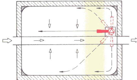
**Fig. 5. Pivoting jet cleaner in a rectangular tank.**
