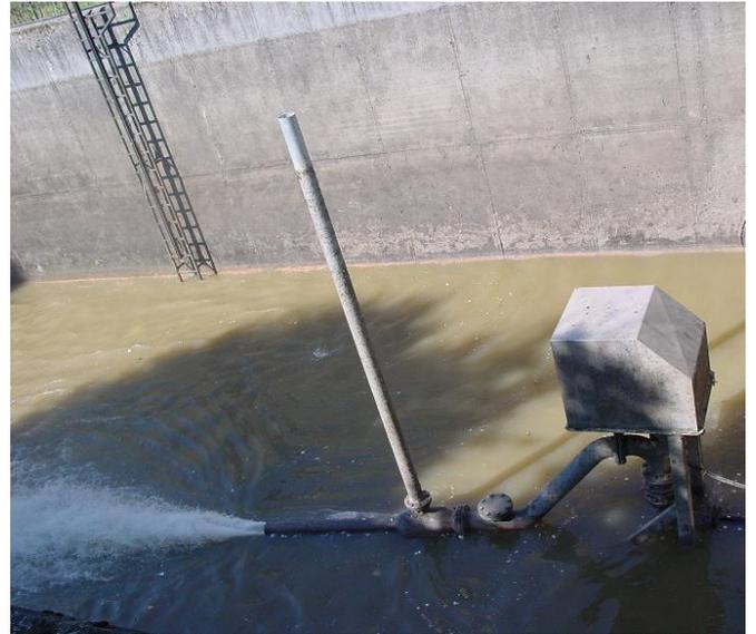
**Fig. 8. Pivoting jet cleaner running.**
