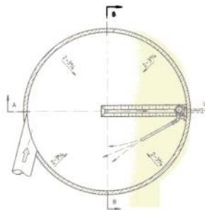
**Fig. 6. Pivoting jet cleaner in a circular tank.**
